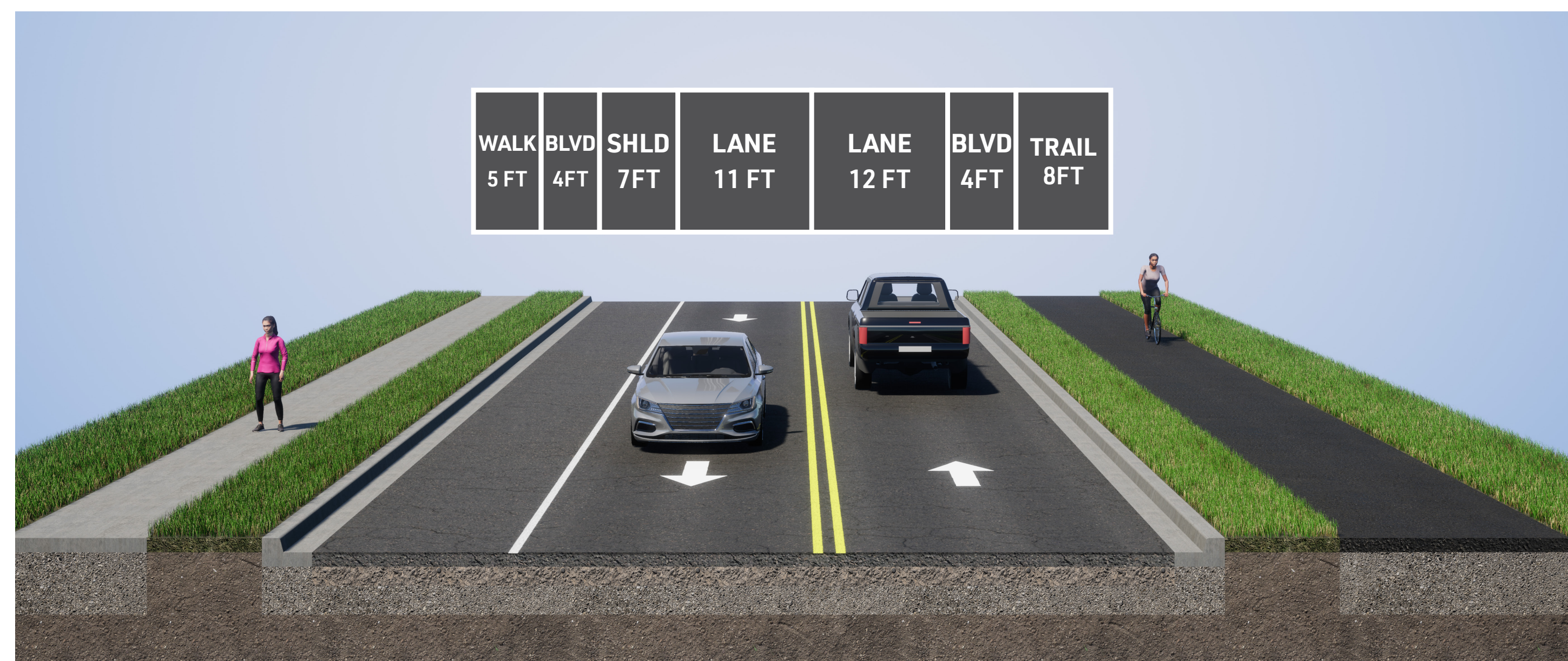
Proposed Butler Avenue Typical Section (Looking East)
